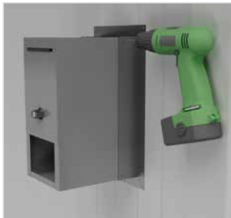
4 Drill 3.5mm pilot holes into the letterbox and screw fix two provided screws each side. Discard angle brackets from screw packet.
