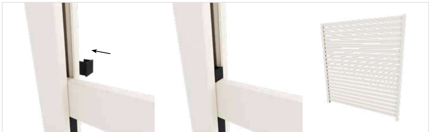
8 Snap in spacer block above first slat into either side of pocket of post. Repeat for all slats.
